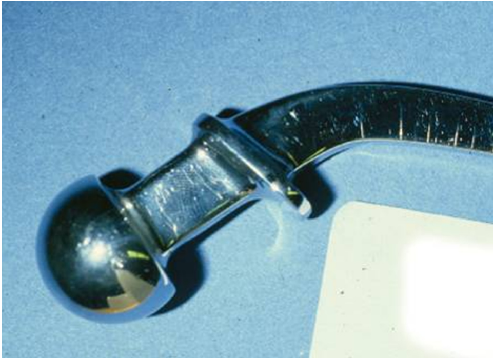
FIGURE 1.4 Femoral replacement part (T28) with stress corrosion cracking. Courtesy of Stanley A. Brown, U.S. Food and Drug Administration.
