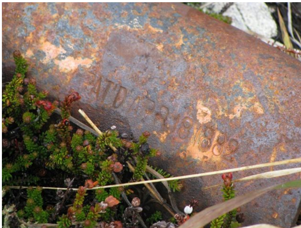
FIGURE 3.6 A ferrous based alloy exposed to the environment since 1882 (note the date on the part). With a cold and dry environment the corrosion process is very slow. SOURCE: University of Virginia Center for Electrochemical Science and Engineering, courtesy of John R. Scully and UVA MSE 3080 class participant.
